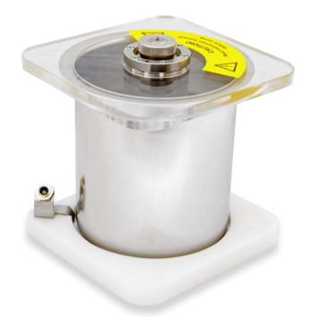
The CP TC12 is used in conjunction with the CPC 100 and CP TD1 to measure tangent delta / power factor and permittivity of insulation liquids, e.g. transformer oil. The three-electrode design with guard allows precise measurement, especially of small losses.
