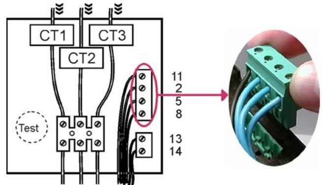
Picture 14: Connections for full equipped device, position of battery and picture of connectors
