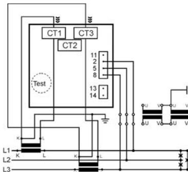
Picture 11: Three phase system (three wire unbalanced - 3u)
