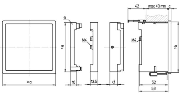
Picture 15: Dimensional drawing EQxx07A and YQxx07A (all dimensions are in mm)
